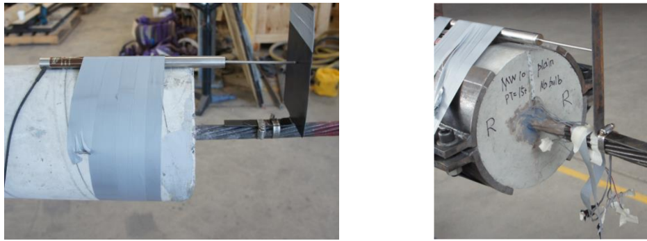
Figure 4: An LVDT monitoring displacement at cable end with and without strain gauges
