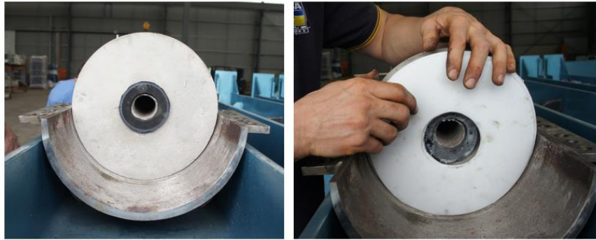
Figure 2: Teflon sheets with Neoprene seal for frictionless shear of the cable
