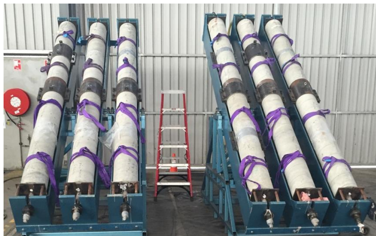
Figure 3: Angled cable grouted samples in 3.6 m concrete cylinder
