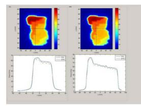
**Figure 2.** Static dosimage acquired using an Electronic Portal Imaging Device (EPID): Treatment planning system (TPS) dosimage (top left) and profile (bottom left) and EPID reconstructed dosimage (top right) and dose profile (bottom right).
