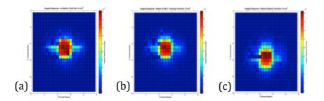
**Figure 3.** M512 array acquisitions,  $(1 \times 1 \text{ cm MLC})$  (a) static MLC, static dosimeter, (b) static MLC, moving platform, (c) moving MLC moving platform (i.e. dynamic dosimaging).
