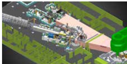
Layout of the Australian Centre for Neutron Scattering. The green shielding to the right contains the nuclear reactor, producing neutrons which are distributed along the beamlines to the instruments. Bilby and Quokka are to the left, Kowari in the centre, Wombat to the top centre, Dingo at the reactor face.
