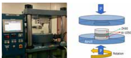
High-pressure torsion apparatus at Hanyang University (left) and schematic of processing (right). Specimens, here magnesium ZK60 and aluminium alloy Al-1050 were sandwiched and processed under pressure P = 6 GPa and up to 10 revolutions.
