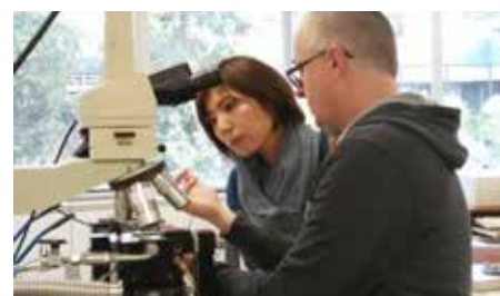
Megumi Kawasaki and Dominic Phelan at the laser scanning confocal microscope with integrated differential thermal analysis, a device for in-situ high temperature studies.
