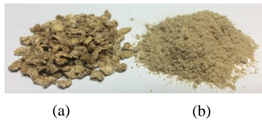
Figure 2: The material used in the experiment is a mixture of coarse (a) and fine (b) particles mixed with the mass ratio of 10:1.
