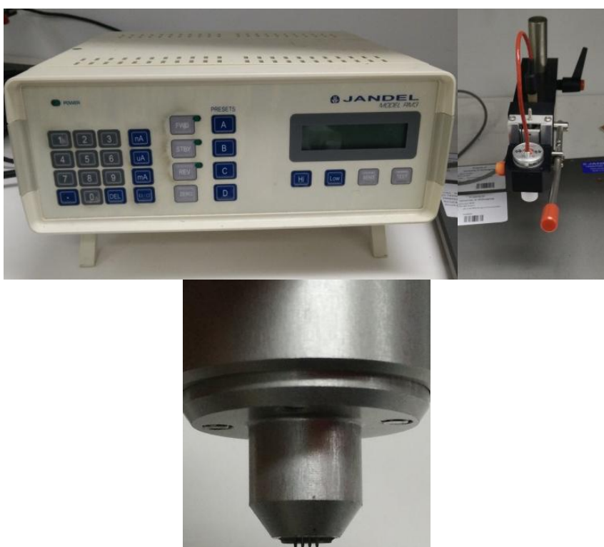
Figure 2.11 Photograph of the Jandel 4 point probe unit (top left), the probe tip mechanism (top right) and a closeup of the probe tip (bottom).
