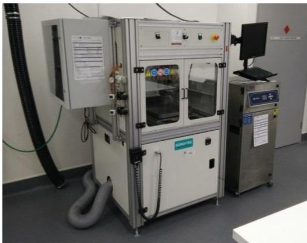
Figure 2.4 Photograph of the Sonotek spraying system.
