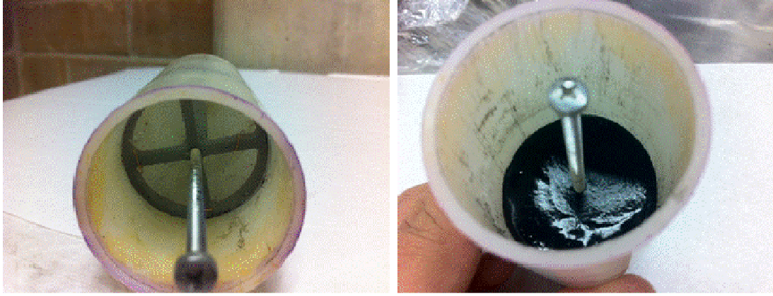
Fig. 1. Modified centrifuge tube before and after test. The photo on the left shows the dewatered cake formed above the centrate in the modified centrifugal test
