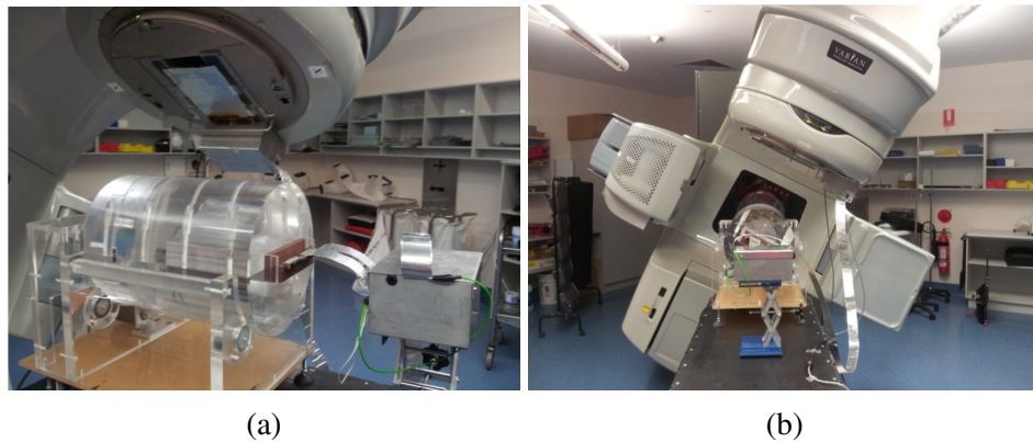
Figure 4.1: (a) The MagicPlate system, showing the MPDM inserted in the rotatable phantom on the patient couch (disengaged; not following the linac head), and the shielded MPTM mounted on the linac head; (b) the system following the linac head.
