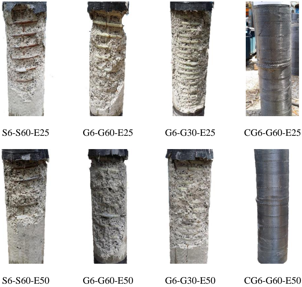
Figure 6.14. Failure mode of tested specimen under eccentric loads
