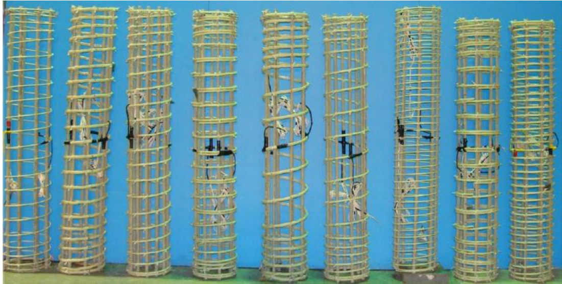
Figure 3.2. GFRP assembled cages 47
