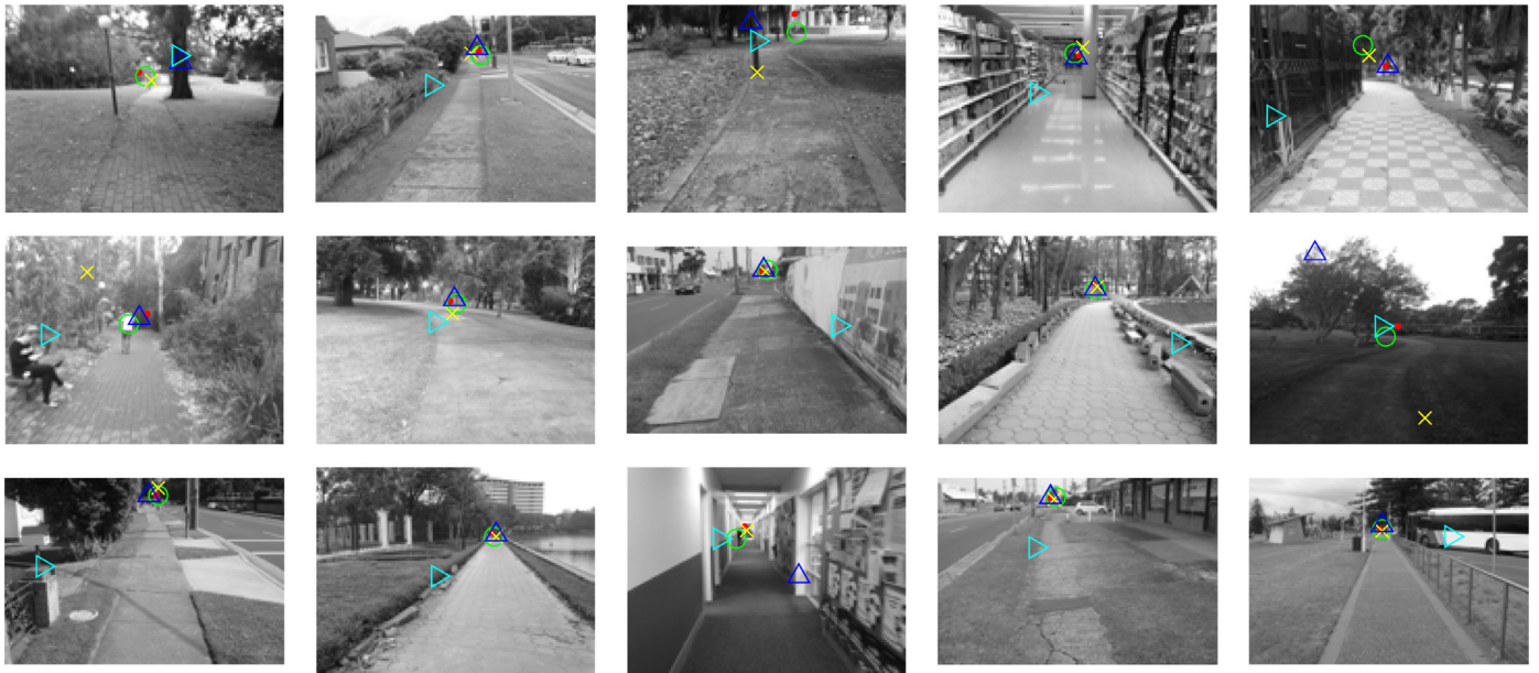
Fig. 6. Visual results of vanishing point estimation. Ground-truth VP: red dot. VP detected by the proposed method: green marker. VP detected by Hough-based method [27]: yellow marker. VP detected by Gabor-based method [16]: blue marker. VP detected by OLDOM [30]: cyan marker. See the electronic color image. (For interpretation of the references to color in this figure legend, the reader is referred to the web version of this article.)
