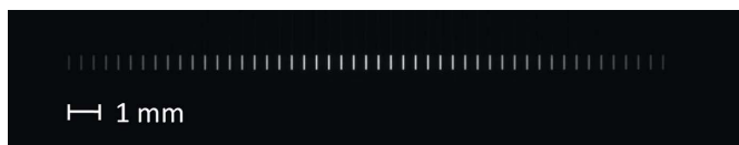
Figure 4 Image of the 20 mm × 520 μm parallel array of microbeams obtained with the FReLoN camera.
