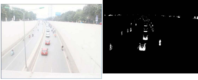
Fig. 2. Background subtraction algorithm a) Original frame, b) Foreground detected
