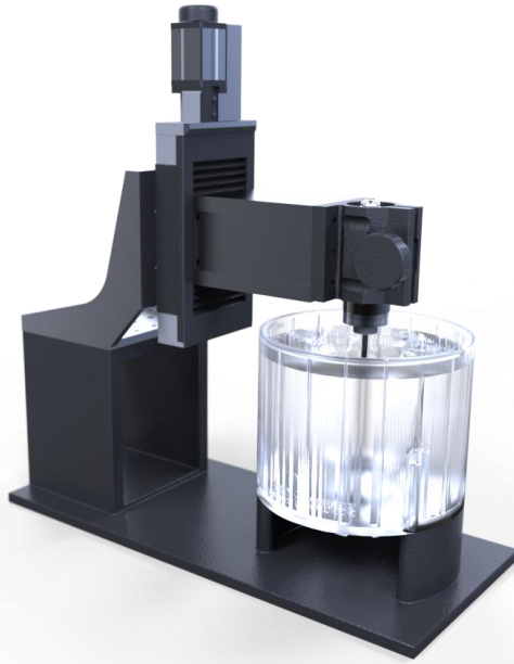
Figure 4. A rendering of the spectroscopic eye plaque verification system
