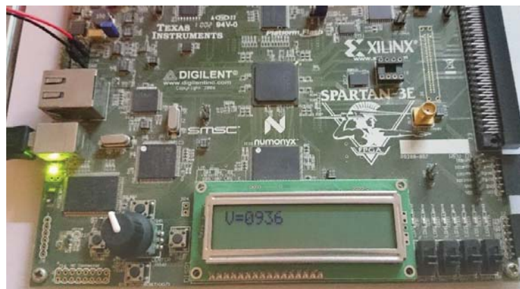
Figure 4-6: ADC module test: LCD displays the actual 14-bit value from ADC (represented in hexadecimal).
