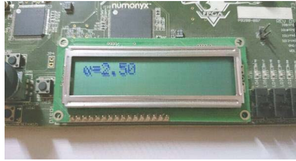
Figure 4-26: Test result of LCD driver module.
