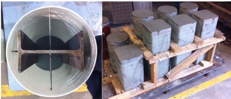
(a) Locating steel I-section
