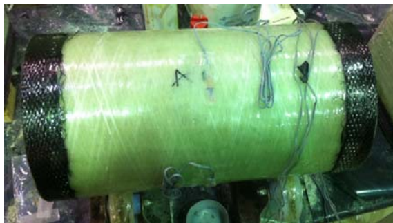
(c) End strengthening with CFRP strips
