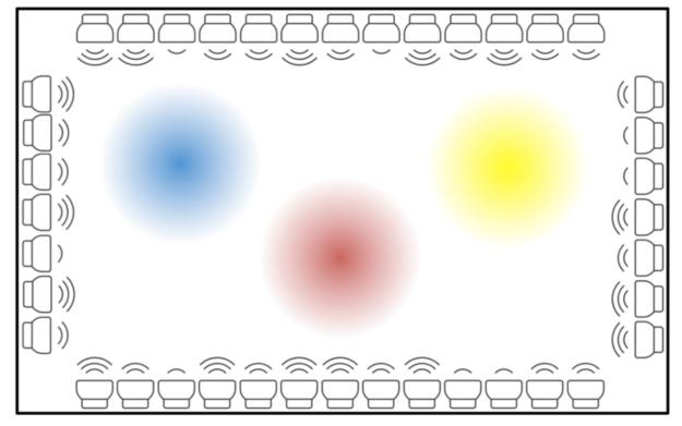
By varying the output of sounds from an array of speakers surrounding a space you can target specific sounds in specific locations. The different sounds here are represented by the different colours. The Conversation, CC BY-ND
