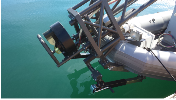
Fig. 2. An ATLAS sonar mounted on the NPS SeaFox USV
