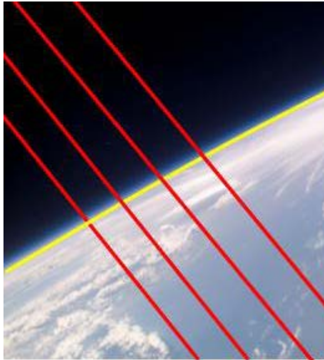
Generic sampling lines that would not be perfectly perpendicular to the horizon, but approximately so due to the discrete orientation classification step.
