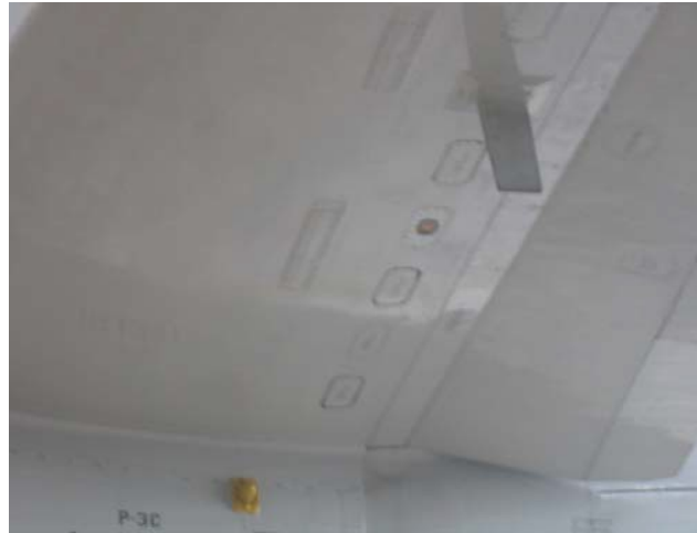
Figure 5. Sensor on Access Panel in Lower Surface of Left Horizontal. Source: Abbott, Columbus, and Beals (2009, 5).
