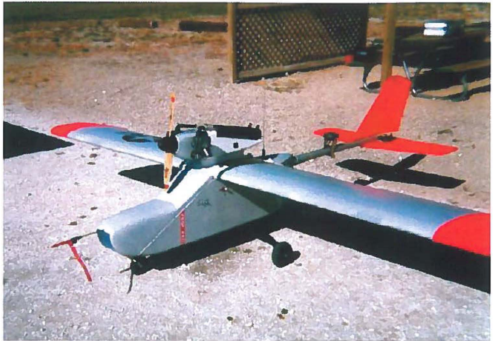
This FROG UAV is used to test experimental avionics software packages. Given the short time students have at NPS, the FROG allows immediate testing of this software.
