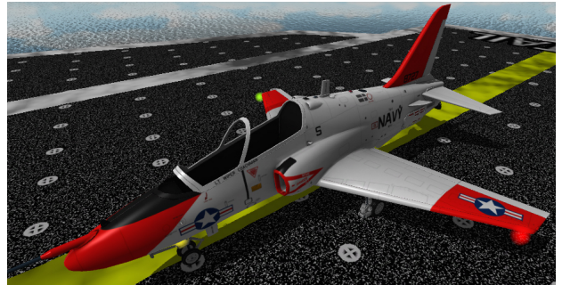
Fig. 7. T-45C 3D model rendered in LSO prototype trainer (size: 110K vertices).
