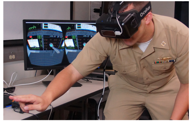
Fig. 11. User demonstrating interaction with LSODS using Leap Motion Controller.
