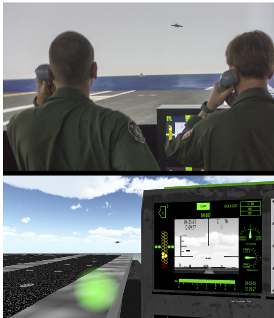
Fig. 16. MOVLAS interface capability with LSODS in both the 2H111 simulator and lightweight LSO prototype trainer.
