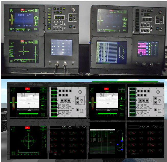
Fig. 10. LSODS comparison between 2H111 simulator (top image) and LSO prototype trainer (bottom image).
