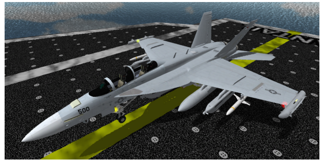
Fig. 8. EA-18G 3D model rendered in LSO prototype trainer (size: 50K vertices).
