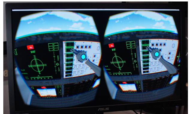
Fig. 12. Stereoscopic displays showing LSODS with LSO's virtual hand.
