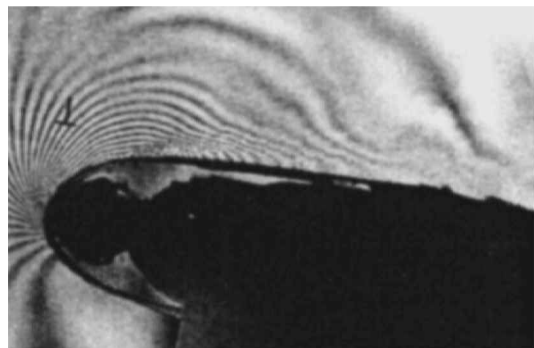
b) Incipient vortex formation, shape 8, \alpha = 12 deg
