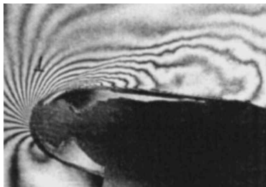
d) Vortex motion, shape 14, \alpha = 12 deg
