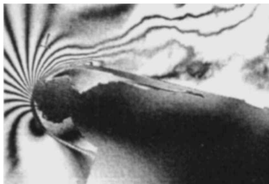
f) Leading-edge separation, shape 18, \alpha = 17.5 deg
