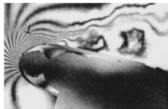
e) Trailing-edge separation, shape 14, \alpha = 17.5 deg
