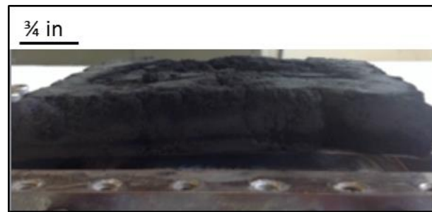
Figure 8. Tridimensional foam generated by the deflector shown in Figure 2f.
