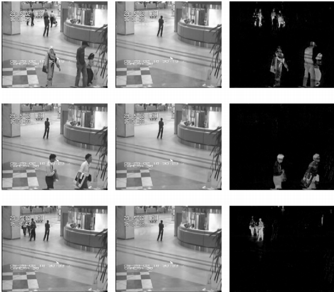
Figure 3.6: RPCA application to video surveillance [32]: (left) sample original video frames in D , (middle) the invariant background recovered by R , and (right) the moving objects (such as people and luggage) captured by S
