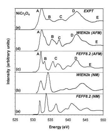
Fig. 4 The oxygen K-edge ELNES of tetragonal NiCr<sub>2</sub>O<sub>4</sub> calculated using non-magnetic (NM) (a, b) and antiferromagnetic (AFM) parameters (c, d) compared with experiment (e).
