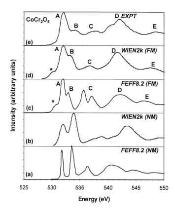
Fig. 5 The oxygen K-edge ELNES of CoCr<sub>2</sub>O<sub>4</sub> calculated using non-magnetic (NM) (a, b) and ferromagnetic (FM) parameters (c, d) compared with experiment (e).
