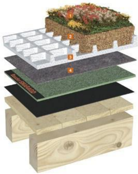
Figure 5.12 Pitched Green Roof. Slope 5° - 15°: ( http://www.bauder.at )
