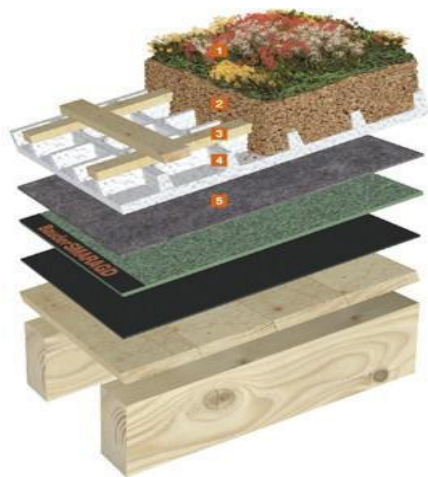
Figure 5.13 Pitched Green Roof. Slope 15° - 25° ( http://www.bauder.at )
