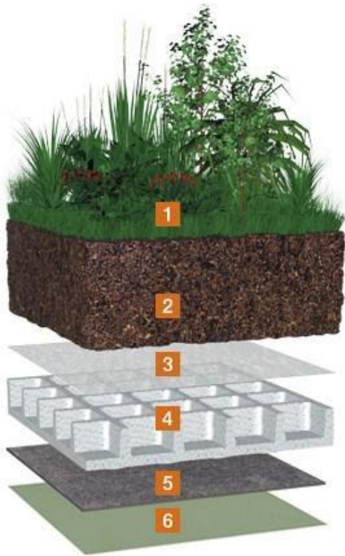
Figure 5.11 “Bauder” intensive Green Roof ( http://www.bauder.at )
