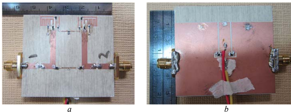
Fig. 2. Prototyped antenna (black wire for ground, yellow wire for controlling varactors and red wire for controlling PIN diodes) a top view; b bottom view
