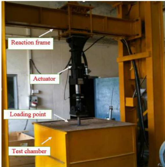
Figure 2 Photograph showing main components of experimental test set-up
