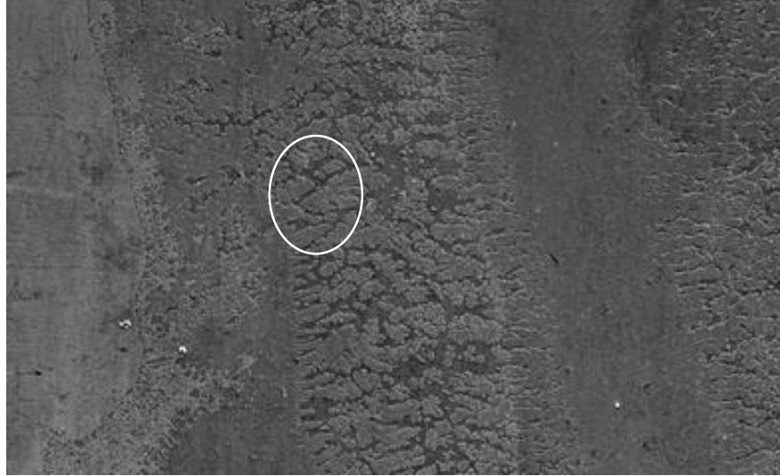
Figure. 4.7 TiNi dendrites growing in both directions
