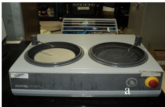
Figure. 3.1 a) Manual paper polishing machine. b) Manual cloth polishing machine
