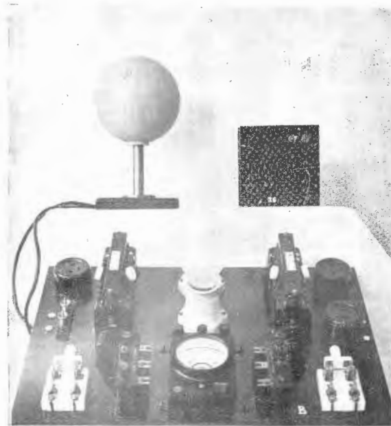
Fig. 6. --Cooling Ball with switchboard and bridge box.
