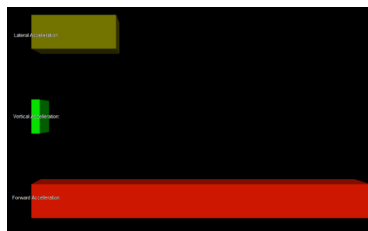
Figure 5 - A screen shot of the magnitude bars of the acceleration (lateral, vertical, and forward). The colours of the bars also vary from green, for small acceleration magnitudes, to red, for large acceleration magnitudes
