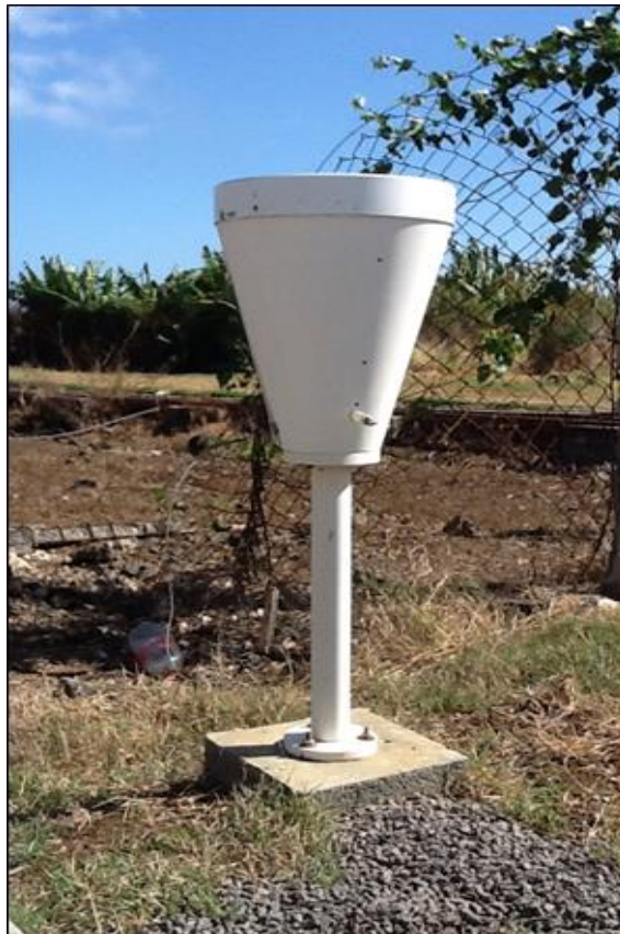
Figure 3-2: Example of the automatic rainfall bucket used by the Mauritius Meteorological Service (MMS) to record rainfall data. Also see Anderson (2012) and Mongwa (2012).
