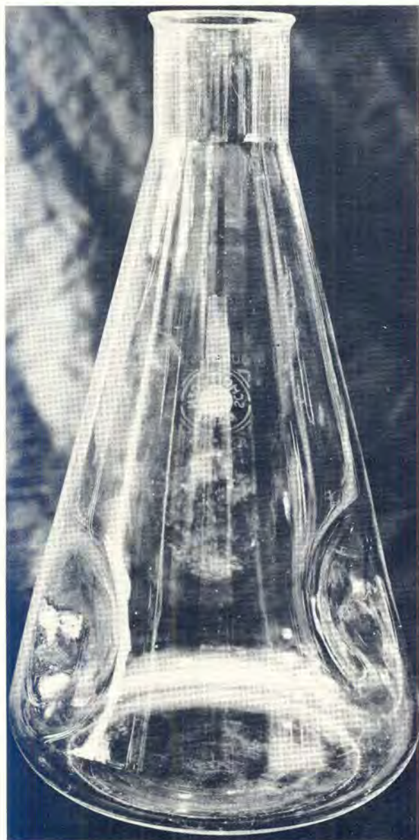
FIG. 10 A 2l flask with indented sides for mixing the worm suspension
