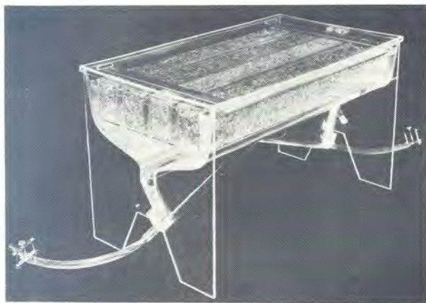
FIG. 1 The hatching chamber (oblique view). The dimensions are: height, 37 cm; breadth, 34 cm; length, 59 cm
