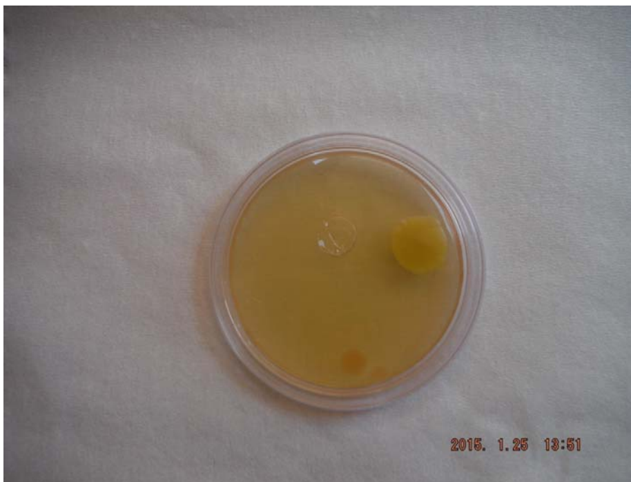
Figure 2: Colony count agar plate with 3 aerobic bacterial colonies
