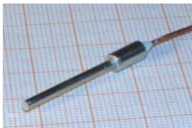
Figure 2 Coaxial thermocouple by RWTH
