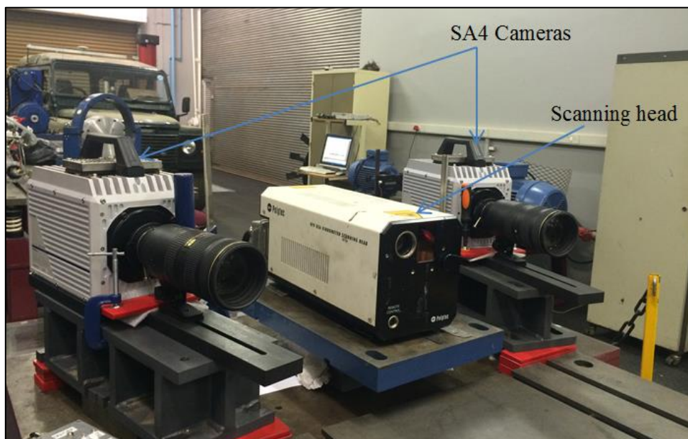
Figure 37: Positioning of the cameras and the laser scanning head
