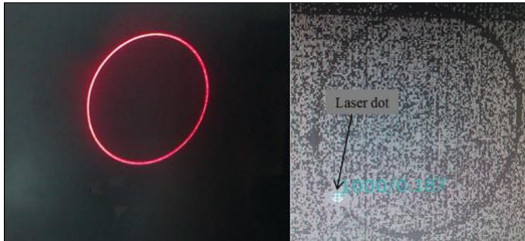
Figure 22: Images of a scanning laser dot focused on a black painted glass panel (10 Hz)
