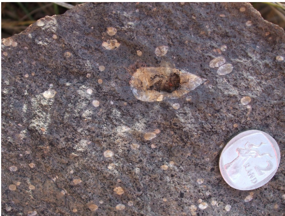
Figure 35. Handspecimen of amygdaloidal rhyodacitic lava. The amygdales are mainly rounded. The spherical characteristic of vesicles is normally associated with pahoehoe lava flows and indicates that gasses were still exsolved when the lava solidified. The coin is 2.3 cm in diameter.
