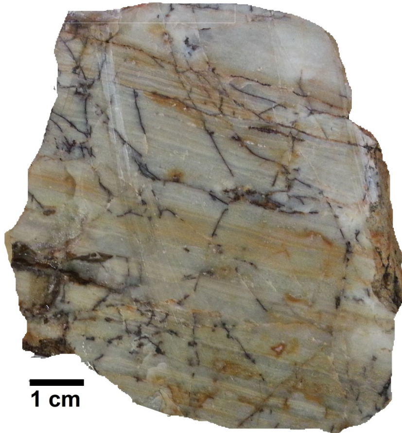
Figure 44. Shows a polished slab of thinly laminated chert. Note the white and reddish parallel lamination.
