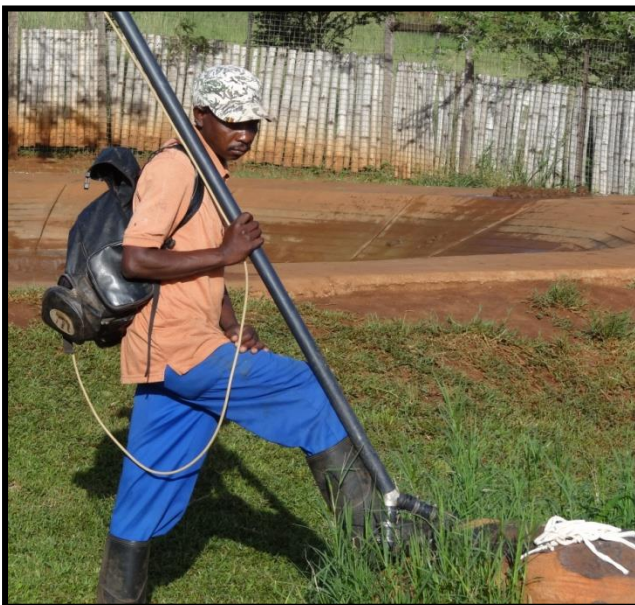
Picture 2: The crocodile stunner consisting of a forked wand and the inverter with battery in the rucksack.
