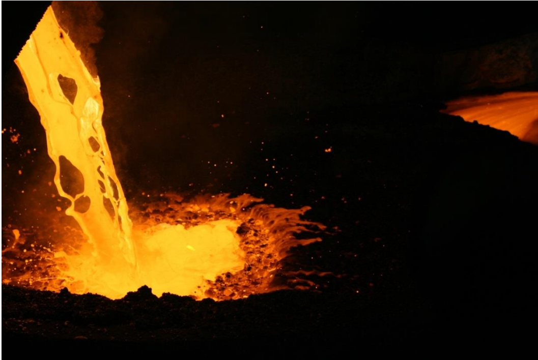
Figure 2: “Follow me” – SiMn metal and slag flowing from launder to ladle and overflowing into a second ladle. Photographer: JD Steenkamp.
