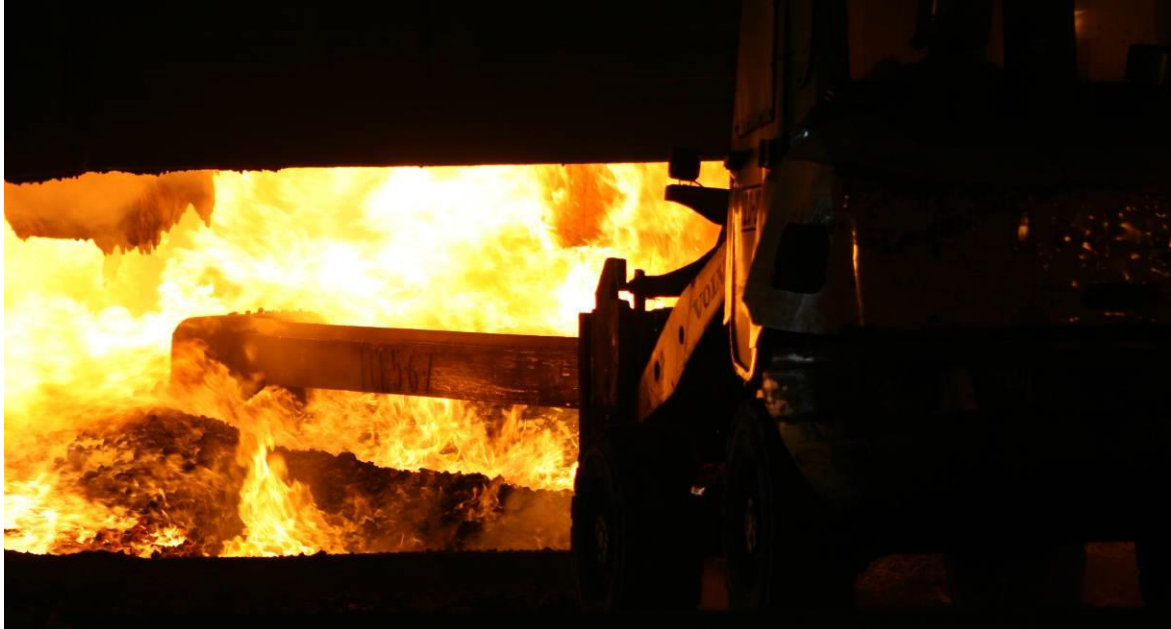
Figure 6: Example of an open furnace utilized to produce SiMn being fed through a feed chute in the roof [16].
