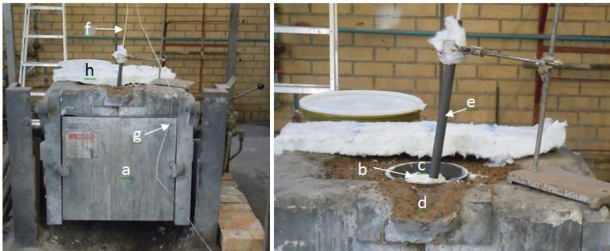
Figure 28: Experimental setup for the preparation of the synthetic slag sample at Mintek with (a) the '50kg' induction furnace, (b) the blend of raw materials, (c) the graphite crucible / susceptor, (d) refractory sand, (e) graphite thermocouple sheath immersed in the slag, (f) alumina thermocouple sheath, (g) type R thermocouple extension wire and (h) mineral wool cover.
