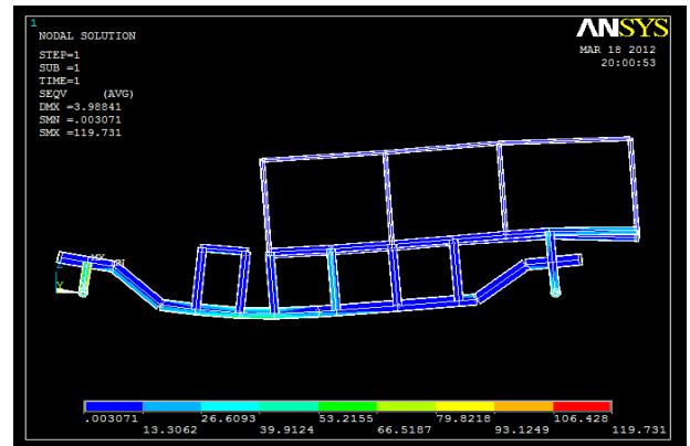
Figure 2 Stress Analysis of Combined Cart
