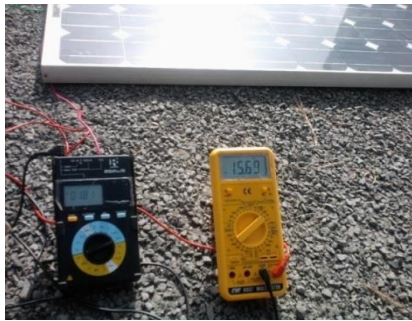
Figure 3 Testing Panel under Variable Load
