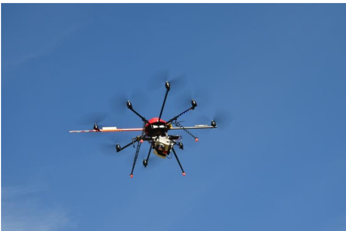
Figure 7 Measurement system consisting of an octocopter carrying an IR bolometer and navigating equipment
