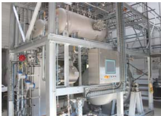
Figure 1 The 58bar pressurized alkaline electrolyzer prototype
