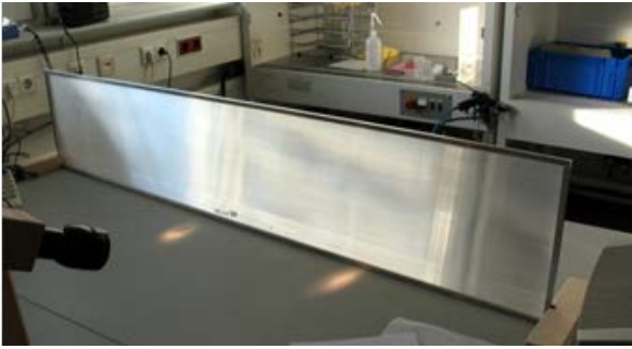
Figure 3 First large-scale prototype with dimensions of 1500 mm x 300 mm x 4 mm for implementation in windows/skylights
