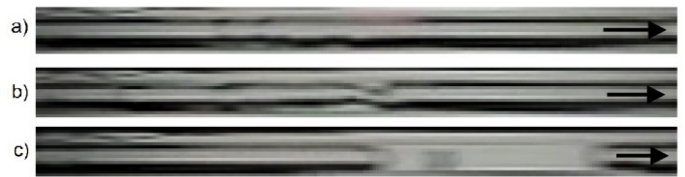
Figure 5 Sequence of flow patterns observed during third mode. a) vapour flow, b) vapour flow with visible tearing areas, c) intermittent vapour flow
