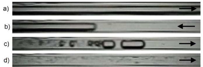
Figure 4 Sequence of flow patterns observed during the second mode. a) vapour flow, b) reversing long vapour slug, c) short vapour slugs with small vapour bubbles, d) bubbly flow.
