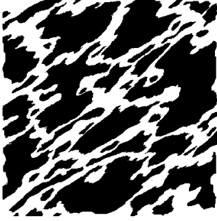
Fig.11. Binary image with porosity of 66% (400x400 pixels) The physical parameters of nickel and air are given below.
