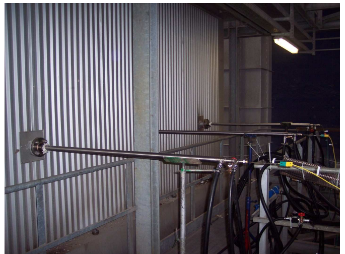
Figure 3 Three suction pyrometers inserted at the top of the rising radiant zone.
