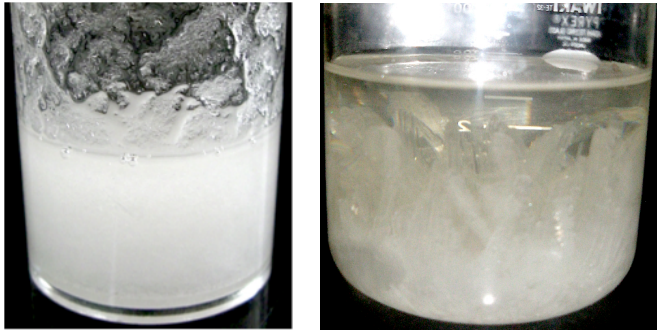
(a) Fine particle slurry of LiBr (b) LiBr crystal lump grown
