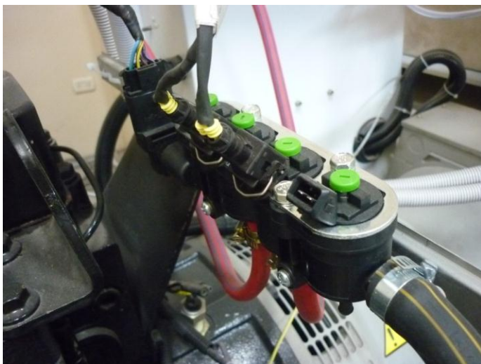
Figure 3 Biogas injectors (dosifiers)
