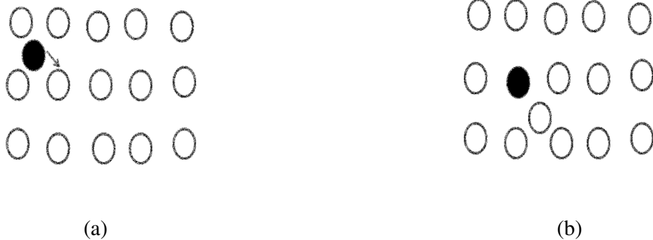
Figure 2.6: Interstitialcy mechanism of diffusion: (a) and (b) are the positions of the self-interstitial before and after diffusion respectively.
