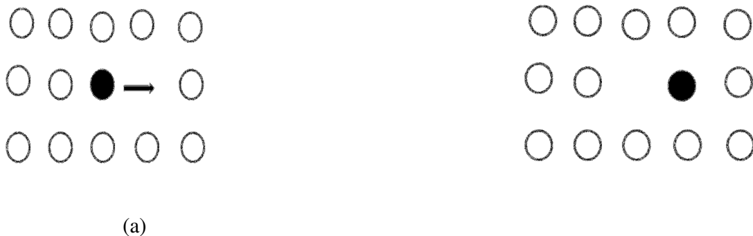
Figure 2.4: A schematic illustration of the vacancy diffusion mechanism: (a) and (b) are the positions of the atom before and after diffusion respectively
